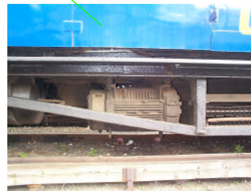
Motor Generator Set
