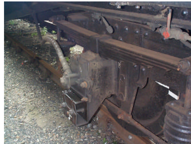
Mechanical drive to de-icer fluid pump (930102)
