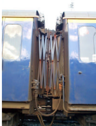
New Gangway, Power jumper side (930202)
