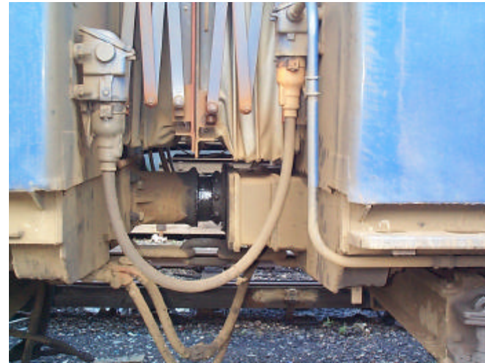
Gangway, close-up of buffer & coupling arrangement (930202)
