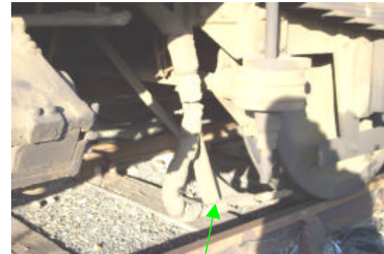
Sandite laying pipe on trailer bogie (No.3 wheel) No.2 vehicle
