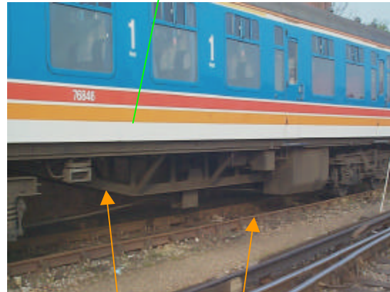
Shoe fuse & AWS receiver
