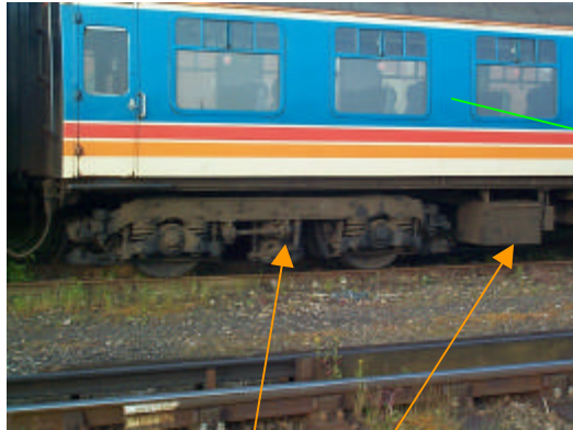
Mk.6 bogie & battery box
