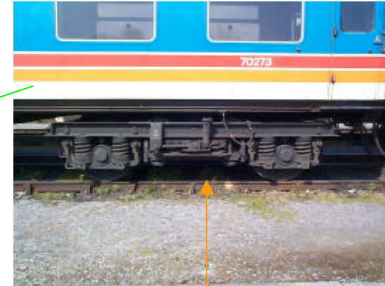
B5S trailer bogie (ex. CI.422 buffet)
