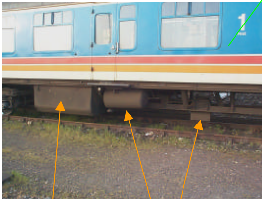
Water tank, Supplementary reservoir & AWS Receiver
