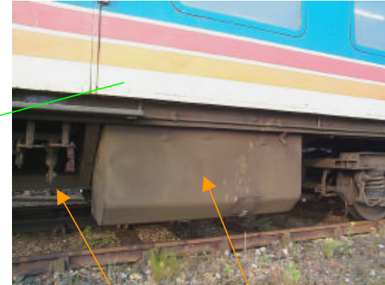
Brake air strainers & water tank
