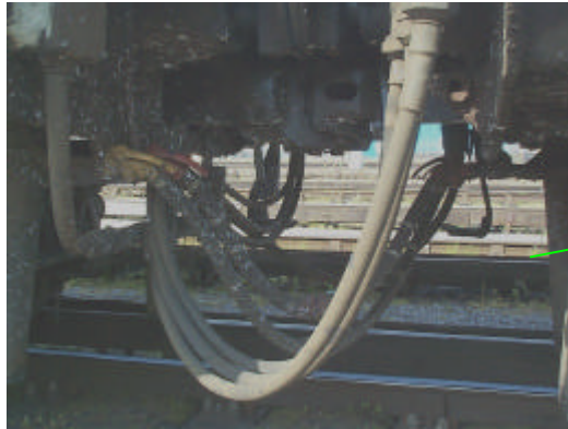
Jumpers connecting to DTC (left) (control side)
