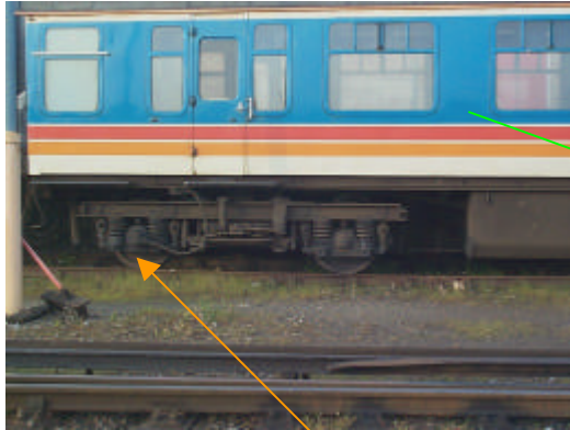
B5S Bogie with speedo generator
