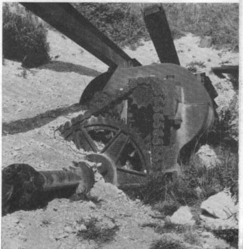
The Whitaker boring machine as it was left at the mouth of the 400-ft. tunnel in 1921. This view is from the back of the machine, the cutting head remaining buried in chalk
