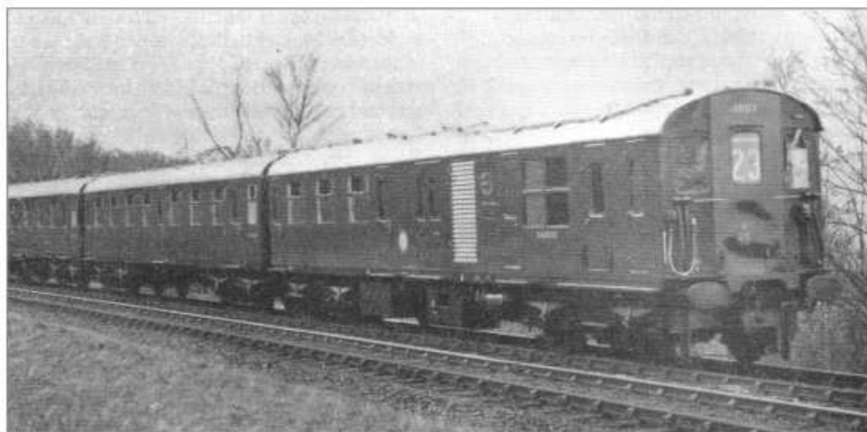
Motor and trailer coaches of new diesel-electric train for the London-Tunbridge Wells-Hastings services
