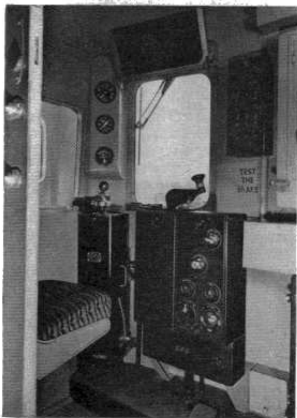
Driver's compartment in motor coach of new L.M.R. electric stock
