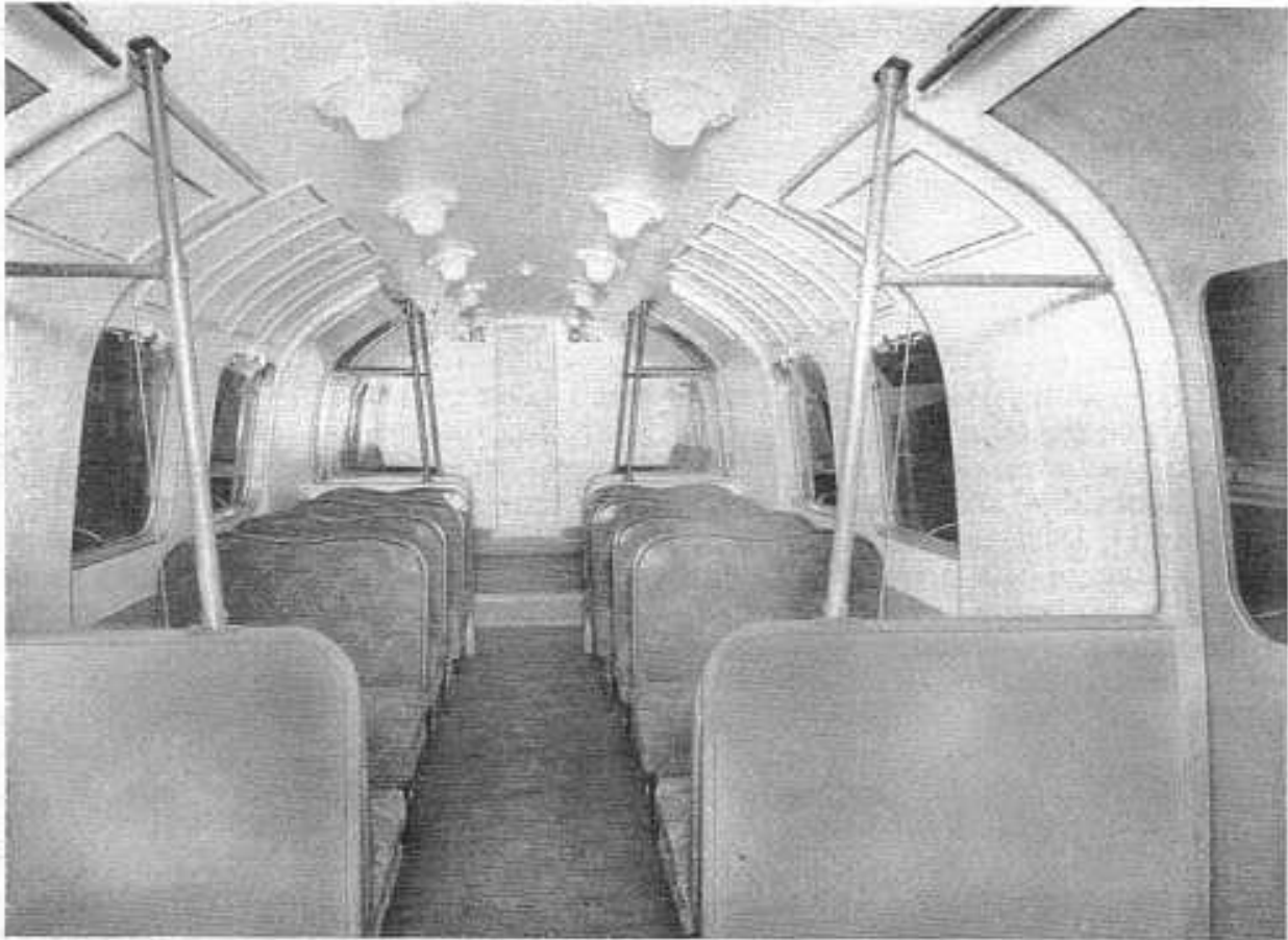
Interior of new all-steel stock with which the Southern Railway replaced in 1940 the original trains of 1898
